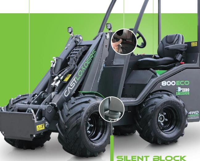
It is equipped as standard with a device that allows greater driving comfort: the Silent Block. This device has been designed to cushion shocks and jerks while driving, especially in rough terrain situations, improving grip and stability.
