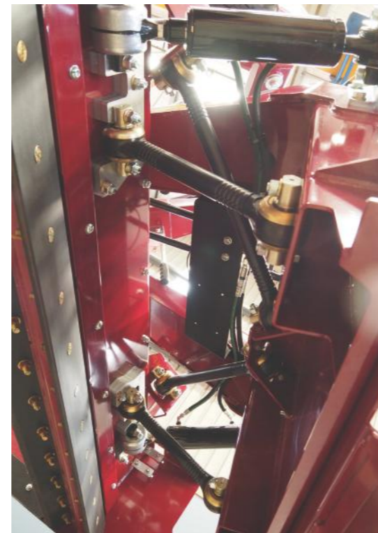
SEALED, GREASEFREE QUADROD® LINKAGE
